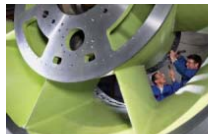
Gas turbine. Working on compressor inlet.
